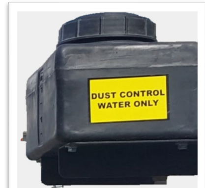
Figure 8: Water tank retrofitted on the Von Arx va 25s
