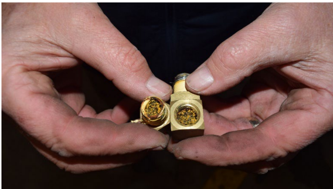
9. Water deposits can clog the valve and prevent flow from the port.
