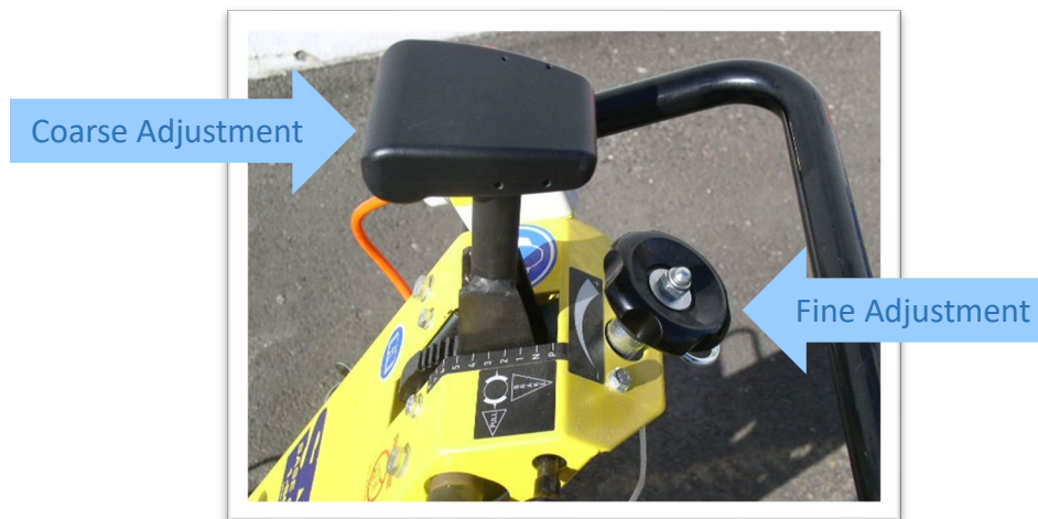
Figure 10: Course and Find adjustments on the Von Arx va25s
