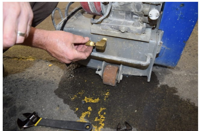
9. Water deposits can clog the valve and prevent flow from the port.
