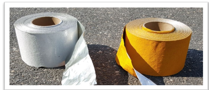
Foil Tabs – can be used as temporary line before permanent marking is applied
