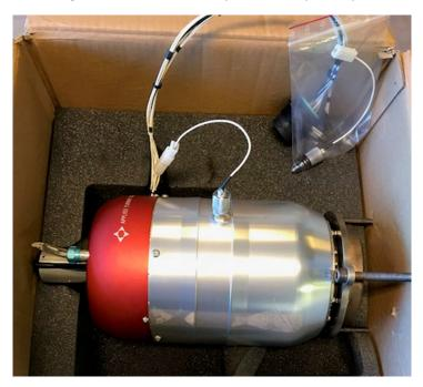
The ignitor is now placed accessible on the side of the jet turbine cover. If an ignitor needs to be changed, a spare ignitor is available on the machine and can be used instead. Changing the ignitor does not require special tools, it can be done by hand following the instructions stated in the products user manual.
