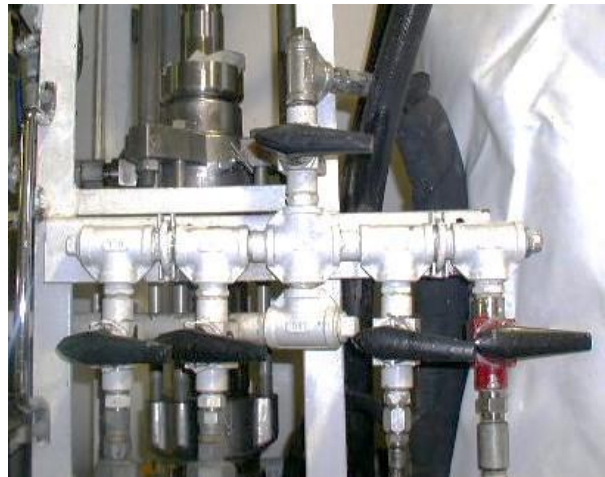
White Supply Valves (Passenger side)
